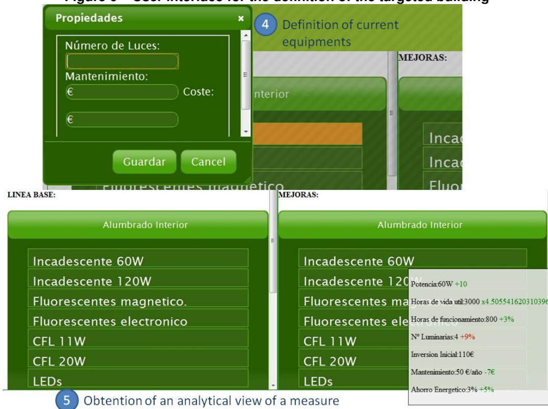
Figure 7 – User interface for the definition of current equipments and an analytical view of a light substitution measure
